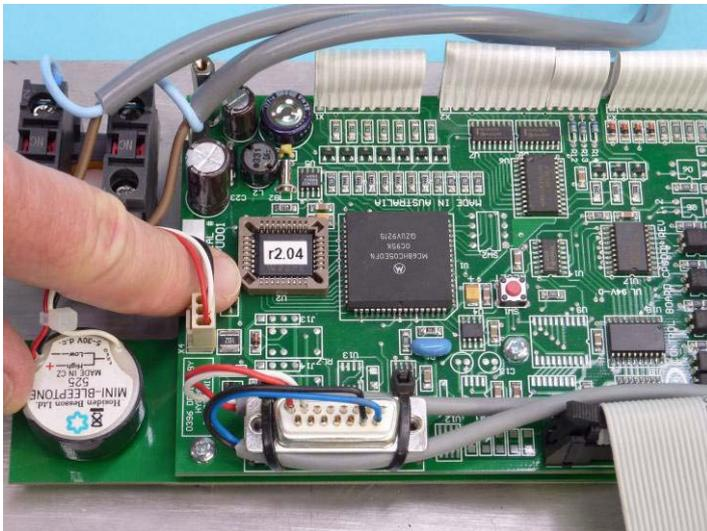
*Check the orientation of the IC.*
