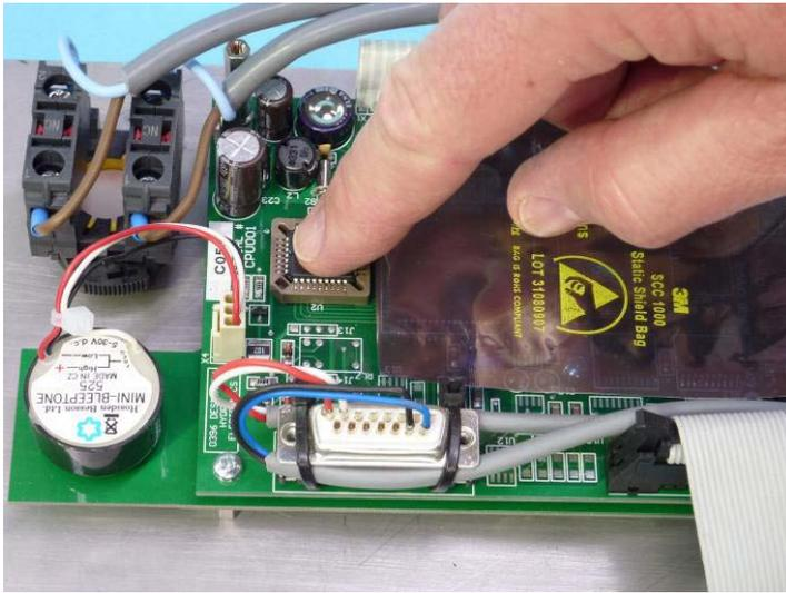
*Press the IC securely into place.*
