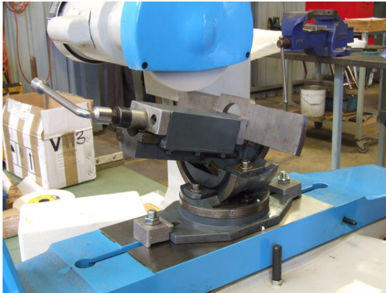
Grinding a Precut Blade in a tilting vice.
