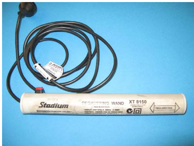
A typical television style "degaussing wand" useful for demagnetising parts
