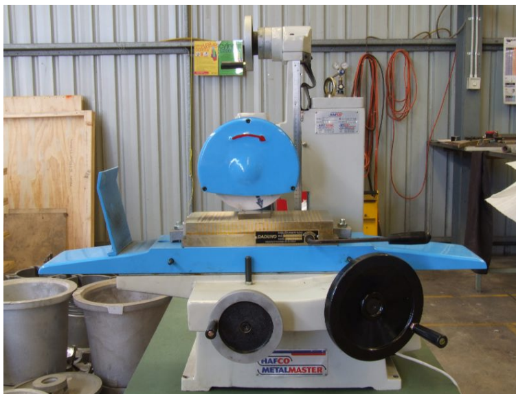
A typical low cost surface grinder and magnetic chuck or table
